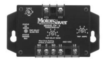
**Model CP-5** is an undercurrent monitor designed to monitor one leg of a three phase system. It is commonly used as a tower monitor on center pivot irrigation systems to detect a stalled center pivot.
